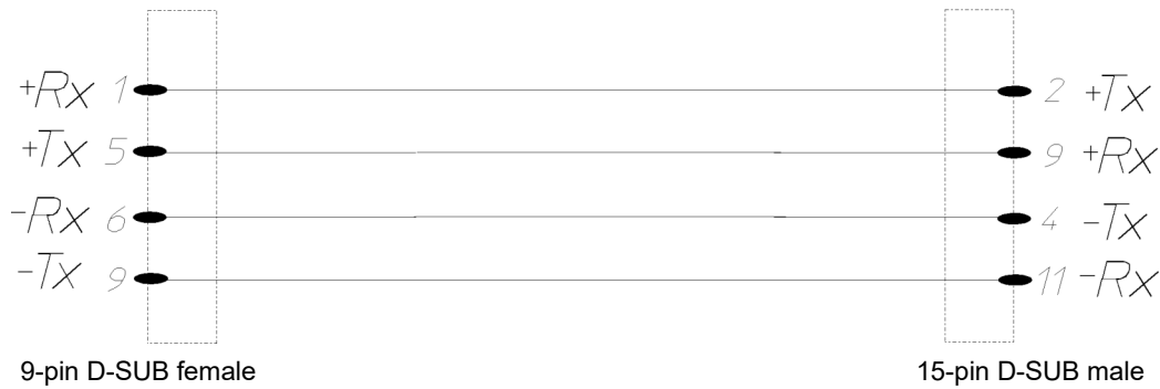
Fig. 4-11 Pin assignment for RS 485 interface cable for Anaprog controllers
