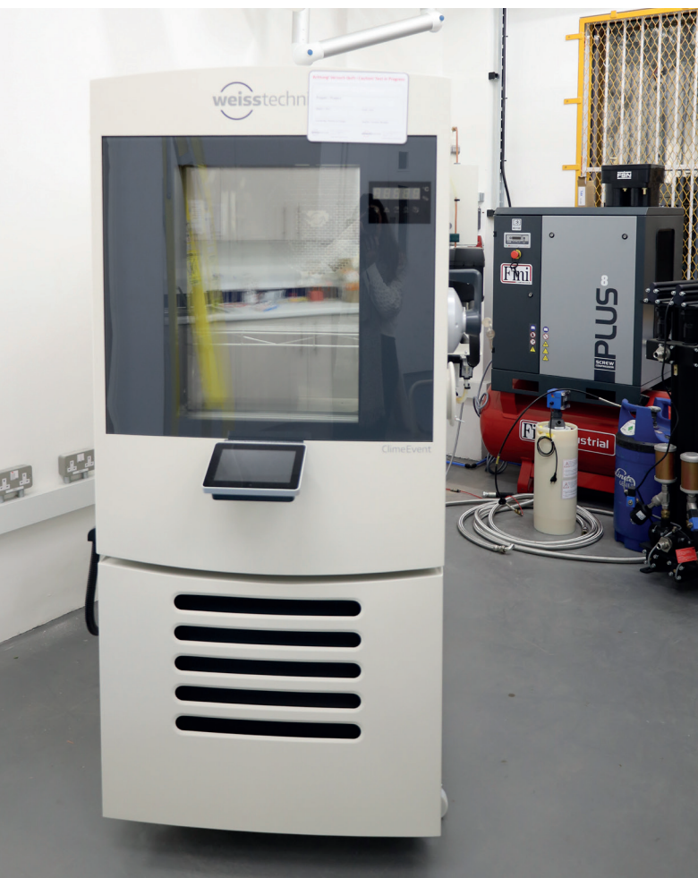
Weiss Technik ClimeEvent C/340/40/3 - Climatic Test Chamber specially designed to include Hydrogen Gas Monitoring.
