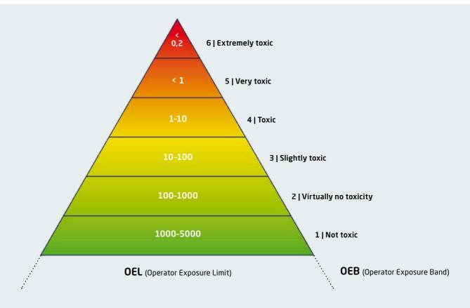
**OEL - Operator Exposure Limit** describes the average concentration of the active substance in µg/m3 within the breathing zone of the operating personnel over a period of eight hours. **OEB - Operator Exposure Band** characterises the extent of the toxicity of the substance on a containment scale from 1 to 6.
