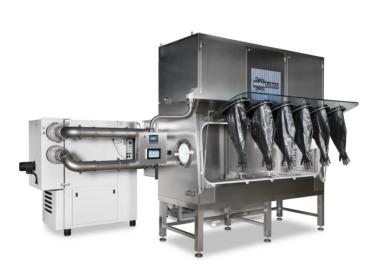
The novel approach of Weiss Pharmatechnik uses an isolator to prepare trays containing the biotechnological substances under controlled clean room conditions with maximum operator and product protection. There is a complete separation from the outside to the inside and vice versa. The highly potent active ingredients cannot contaminate people or the environment, and the product cannot be contaminated by germs.
