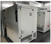
The ClimeEvent climatic test chamber is a multi-functional system in which any climatic conditions can be reliably set. It features low power consumption and whisper-quiet operation. On request, safety measures can be carried out in accordance with the ATEX directive. To prevent condensation during operation under high humidities and temperatures, the
