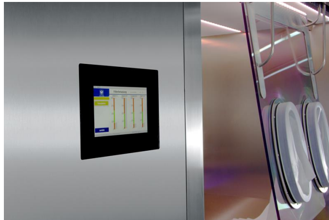
Touch display with graphical representation of filter loading.
