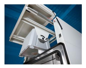
This allows their effects on the test specimen to be examined under laboratory conditions and the ageing caused by solar irradiation, temperature and humidity to be determined. This enables reproducible measurements under defined, continuous conditions, independent from day and season.
