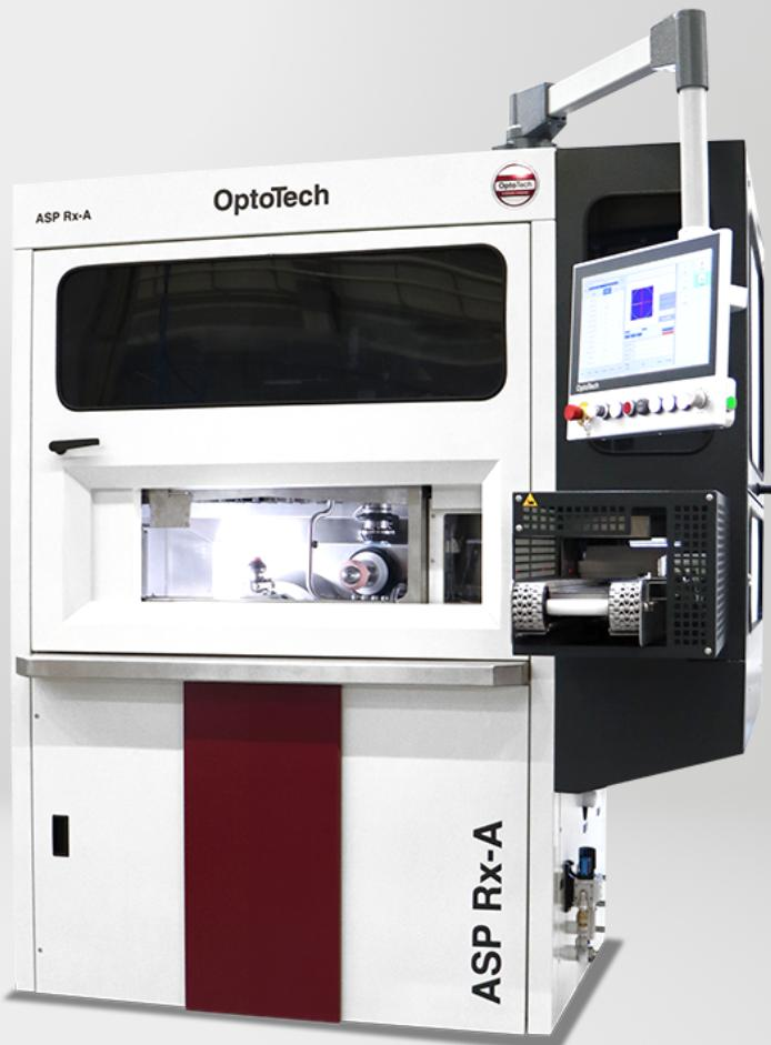
The OptoTech Digital-Surfacing-Polisher ASP Rx-A is designed for full automatic high speed polishing of one toric/atomic or backside progressive mineral lens. Round, oval, or lenses of any other shape can be polished.
