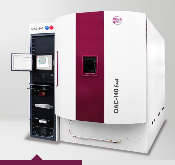
The OptoTech OAC-140 Fast evaporation coater is used for the application of high quality anti-reflective (AR) coatings and clean coats (CC) on ophthalmic lenses. The OAC coating system is characterized by the product quality for which OptoTech is known, ease of use, and exceptional reliability in the daily production operation.
