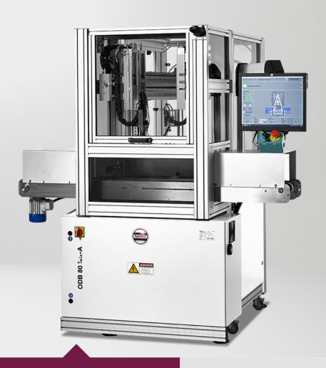
The OptoTech auto de-blocker ODB 80 Twin-A is designed for professional fully automated alloy deblocking. The machine allows uninterrupted de-blocking with no downtime.
