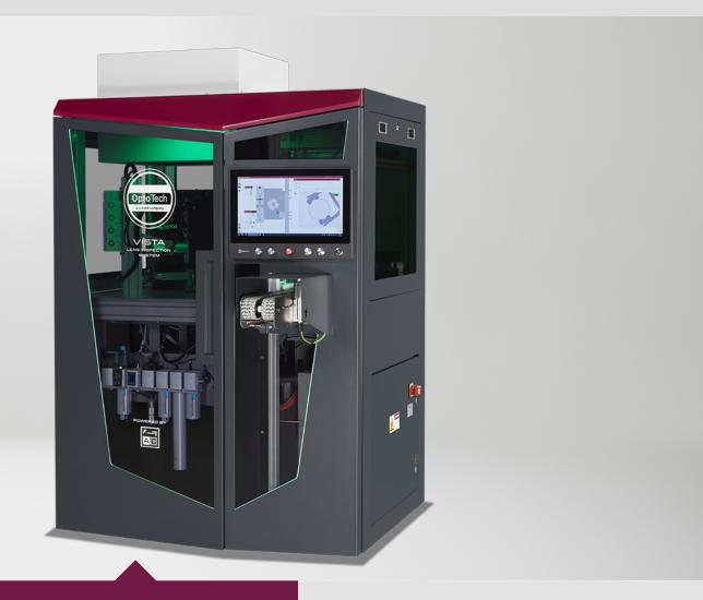
The VISTA is especially designed for detecting and localizing defects on ophthalmic lenses. Detects a comprehensive range of different defect categories. Big Data collection integrated.
