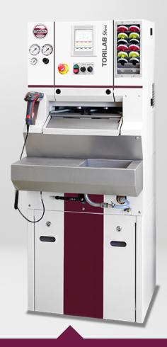
The OptoTech Torilab Store is a 2 spindle machine for polishing toric, spheric and freeform design lenses with only a handful of OptoTech new developed flex tools. The tools have an excellent tool life time so the consumable cost for operating a Torilab Store will be extraordinary low.
