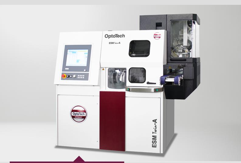
The new digital surfacing machine ESM Twin-A is the ideal complement to our FLASH Twin-A. Due to the usage of 2 milling spindles the ESM Twin-A is able to simultaneously process 2 freeform lenses. Considerably increased speed of the tool spindles, combined with a high-class drive concept, leads to significant improvements in quality and quantity.
