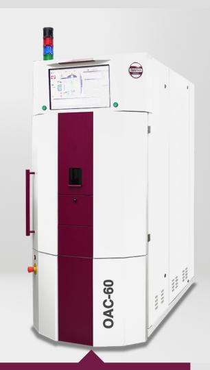
The OptoTech OAC-60 evaporation coater is used for the application of high quality coatings like anti-reflective (AR) coatings and clean coats (CC) on ophthalmic lenses. It is the ideal coating unit for low volume and flexible lens production. The OAC coating system is characterized by the product quality for which OptoTech is known, ease of use, and exceptional reliability in the daily production operation.
