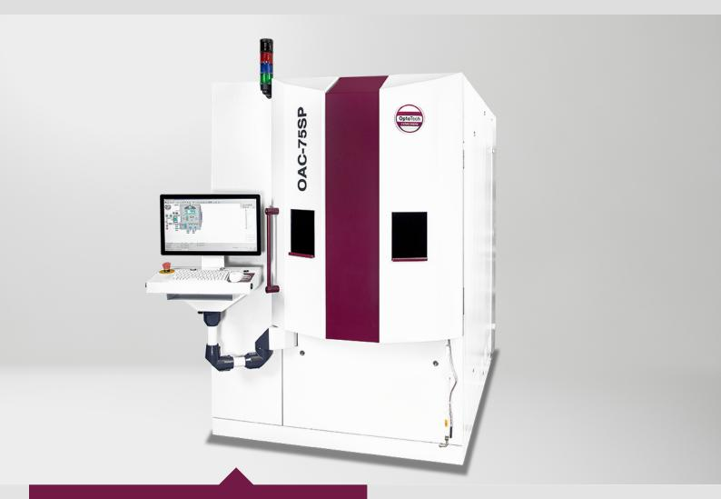
The OptoTech OAC-75SP is one of the most flexible coating machines on the market. This evaporation coater is used for the application of high quality anti-reflective (AR) coatings, clean coats (CC), mirror coats as well as tinted coats on ophthalmic lenses. The OAC coating system is characterized by the product quality for which OptoTech is known, ease of use, and exceptional reliability in the daily production operation
