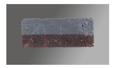
Cross section of a cascade (aluminium-copper connection)
