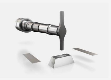
Bending horns are often used for welding spots difficult to reach. In contrast to a standard sonotrode producing longitudinal oscillation, the bending sonotrode is induced to generate flexural oscillation in the center by the vibration oscillator system.
