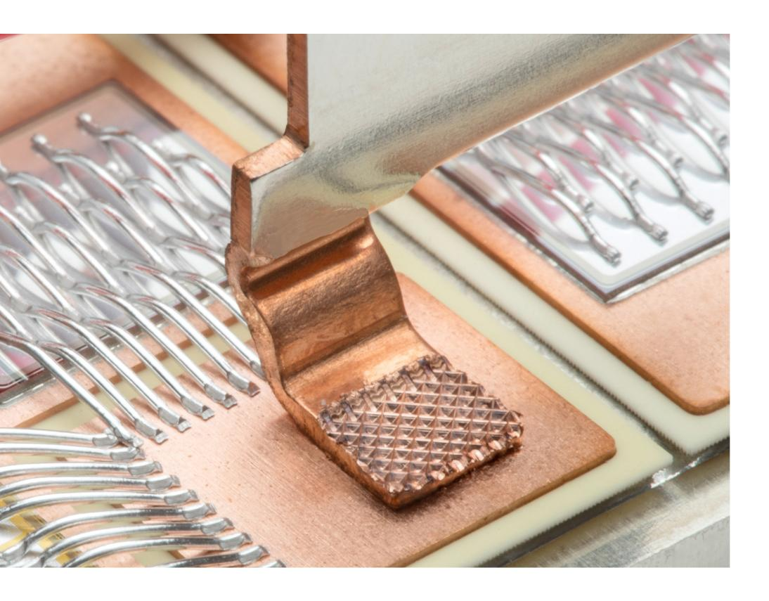
In power electronics, high-performance modules such as IGBTs (Insulated-Gate Bipolar Transistors) or IPMs (Intelligent Power Modules) are increasingly produced by ultrasonic welding. The material-locking connection leads to a significantly reduced power dissipation at the contact points, which increases the electrical efficiency and minimizes the cooling effort. Tests have shown that ultrasonic welding joints significantly increase the service life of the modules.
